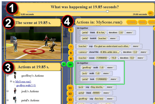
Figure 2. The History tool interface: (1) Time Slider for scrubbing through time, (2) Scene Viewer shows the scene at the selected time, (3) Current Actions Pane shows what actions characters did at the selected time, and (4) Annotated Code View selects the executing line of code, affords block and statement playback and navigational controls.
