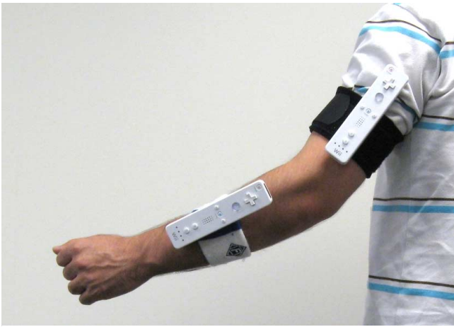
Figure 5. Detecting elbow flexion and extension with Wii remotes. The Wii remote on the upper arm detects and cancels out the compensation by the rest of the body.
