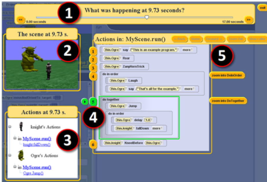
Figure 3: The Output History Explorer Tool Interface. (1) Time Slider for scrubbing through time, (2) Scene Viewer shows scene at the selected time, (3) Current Actions Pane shows what actions characters did at the selected time, (4) Annotated Code View highlights the executing line(s) of code and affords block and statement playback, and (5) Navigation controls for zooming blocks and methods.
